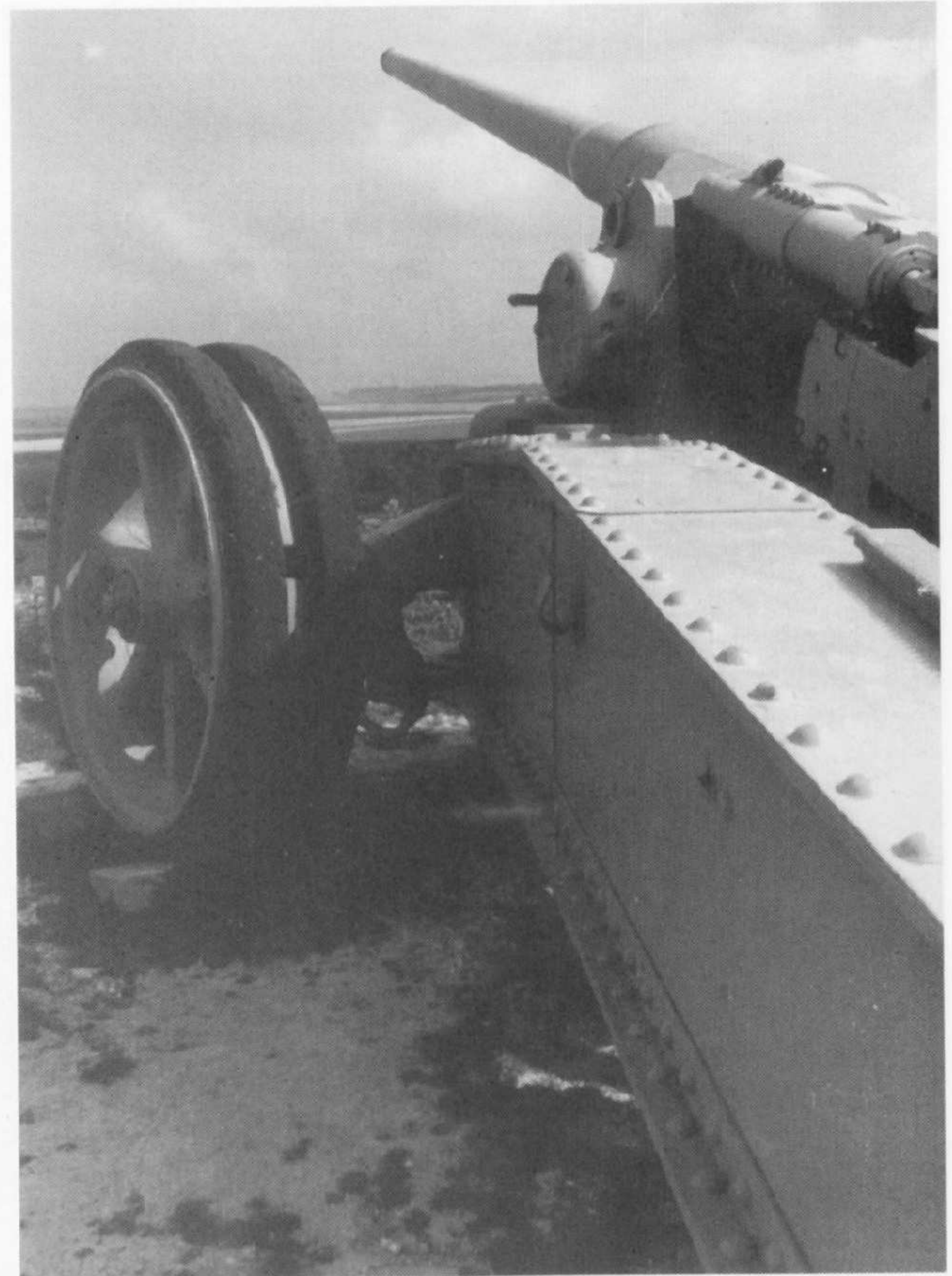
Right: This Field Cannon 418 (f) is in position, with its barrel at its highest elevation of +35 degrees.
