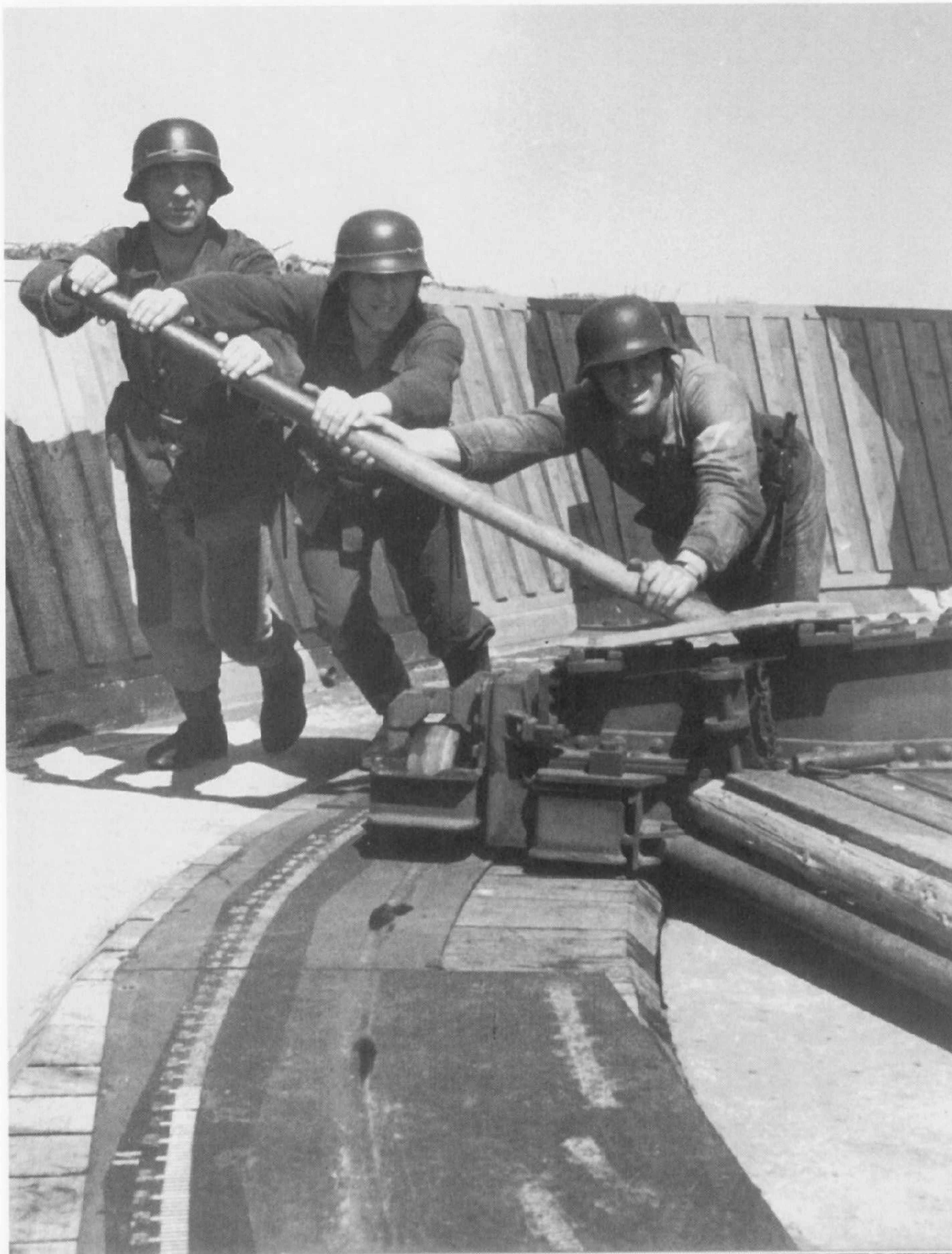
Left: Setting the traverse of the field cannon was hard work, what with the gun weighing 10,750 kilograms. The traversing gunners had to push the gun to the ordered traverse setting with a rod. Here the degree numbers have been painted on the surface of the gun bed. (BA)
