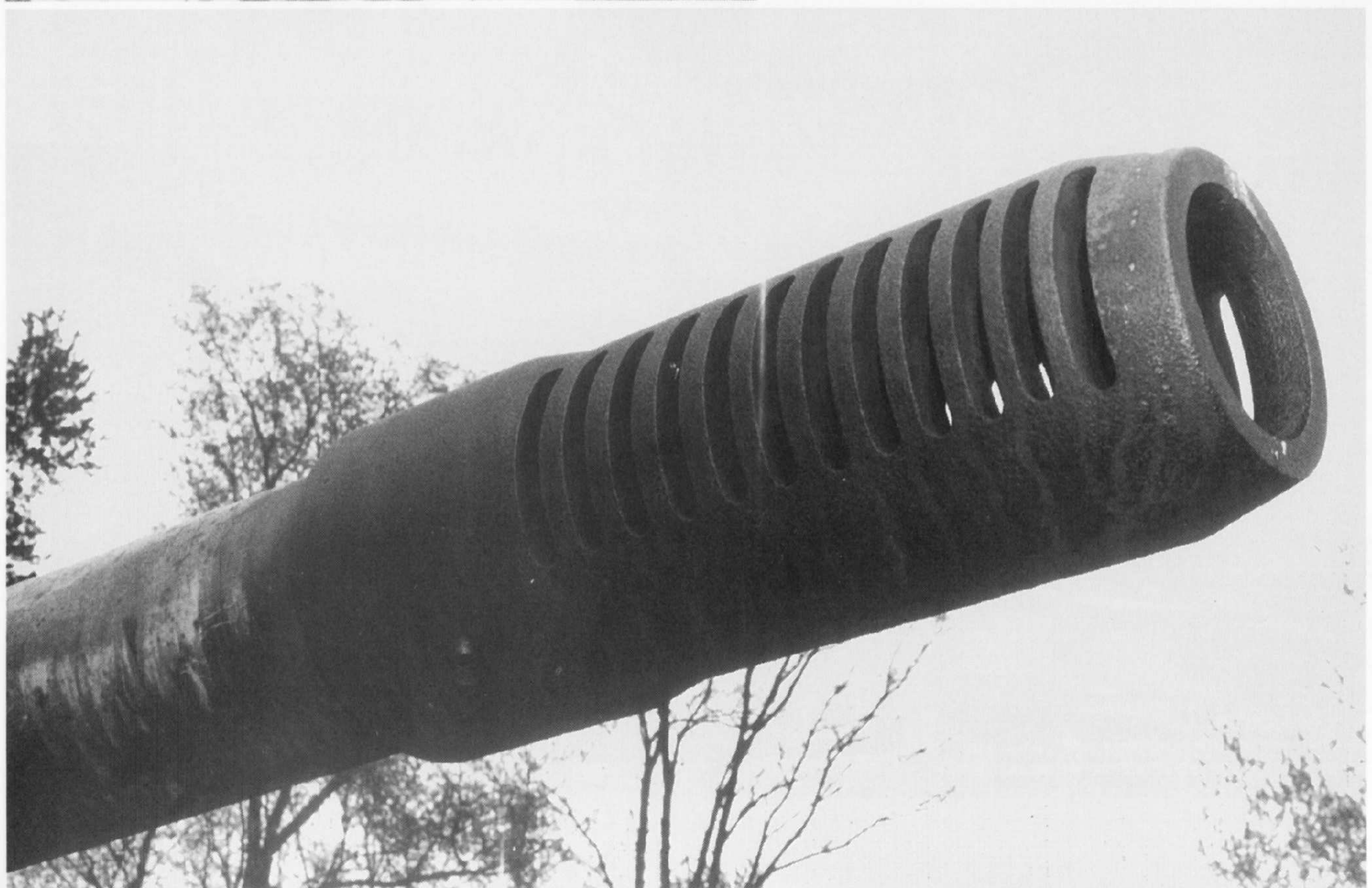
Below: The muzzle brake with its twelve side louvers on either side braked the recoil of the gun when firing by means of a flange, arched toward the back, in front of every opening. In the moment when the shell passed the muzzle brake and thus closed it off, the powder gases were forced out the side louvers and directed backward. Thus the recoil of the barrel was braked and partly eliminated.
