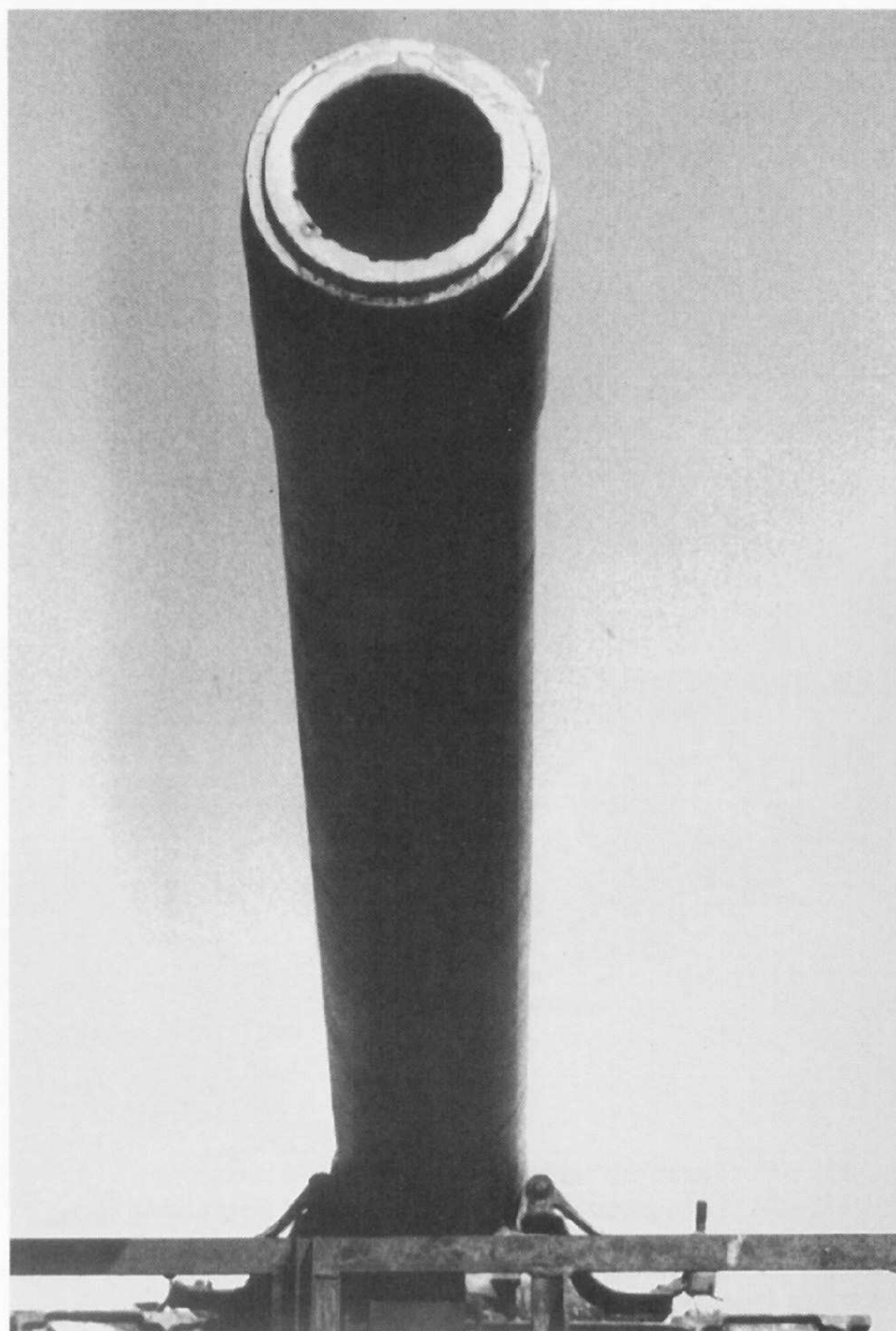
Above: The mouth of the barrel of the K 5, over 21 meters long, with twelve riflings. The inner barrel can be seen protruding slightly from its mantle.
