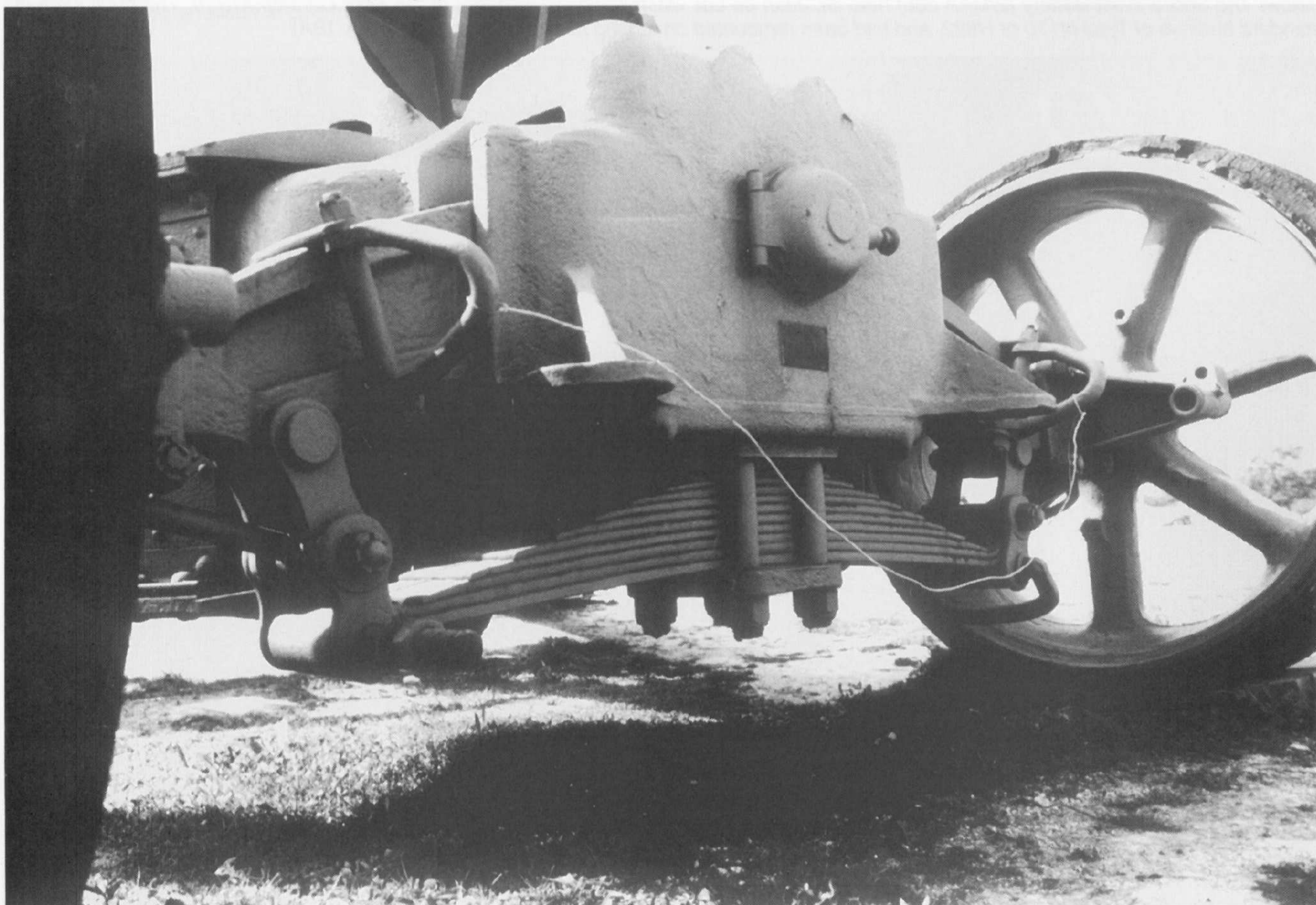
This Field Cannon 418 (f) stands in an open field position. The pair of front wheels were pushed between the mount spars.
