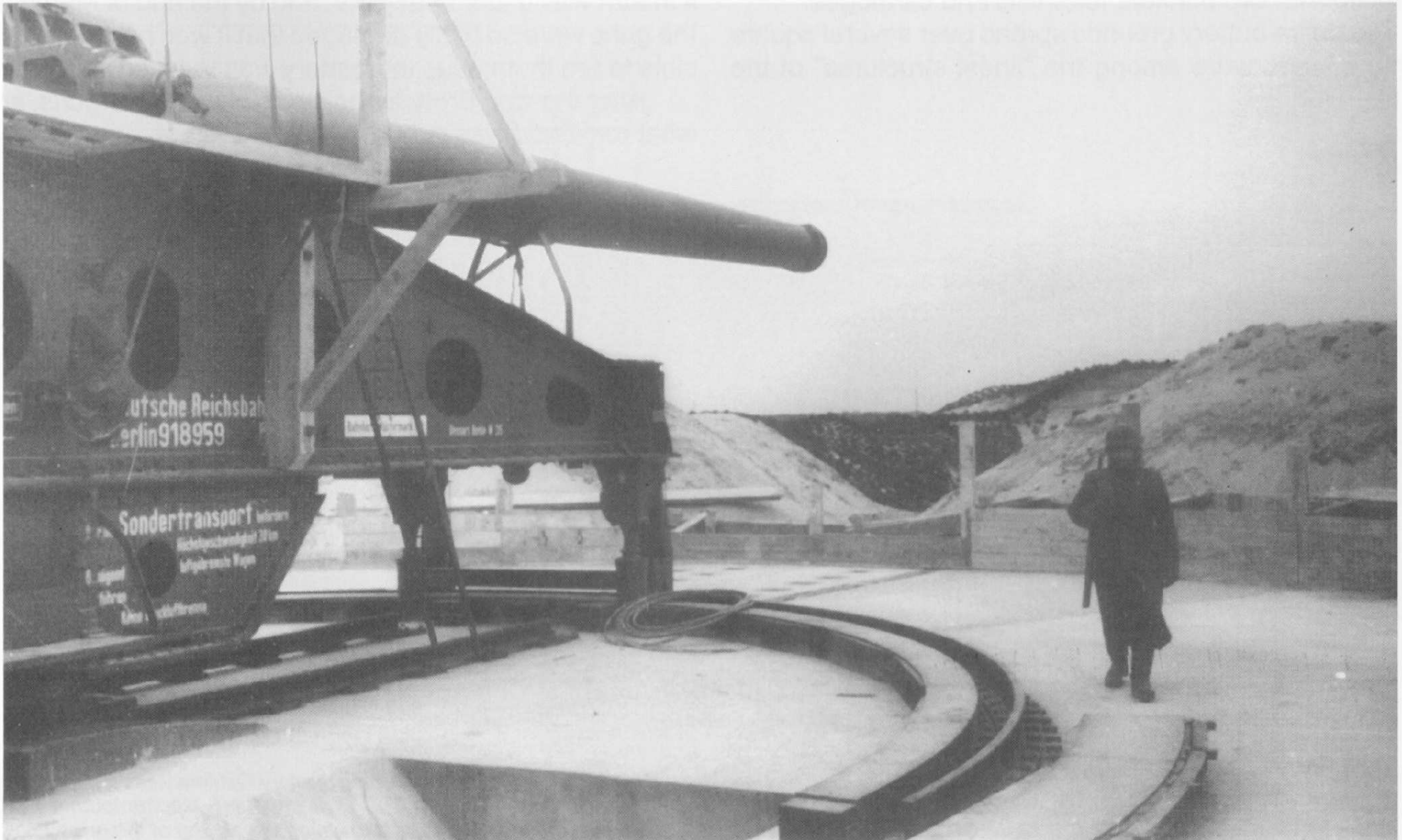
A 34 cm railroad cannon in its bed at Plouharnel.
