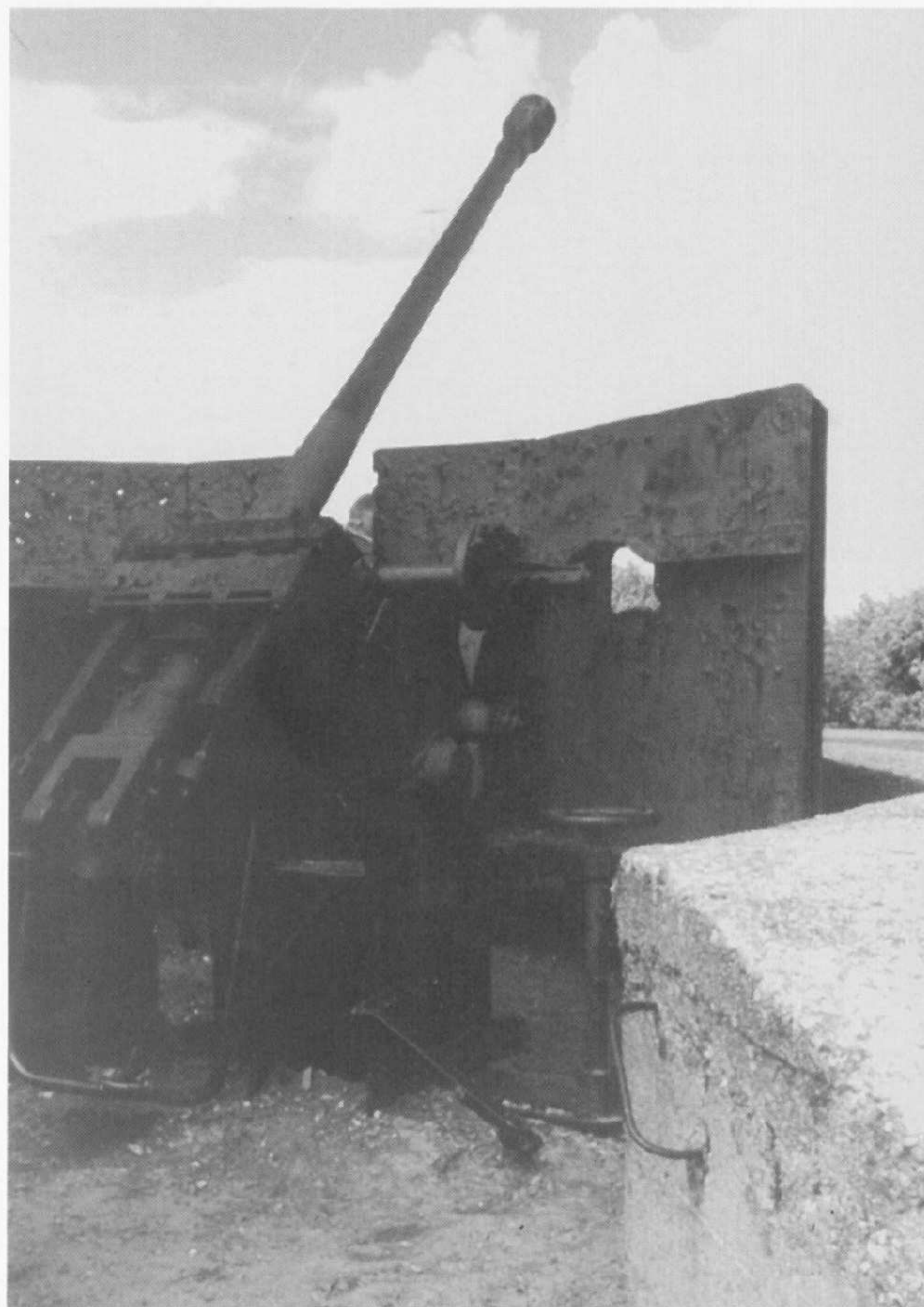
Right: A 5 cm KwK L/60 of Resistance Nest 5 near La Madelaine in Normandy. The barrel is set at its maximum elevation angle of + 43 degrees.
