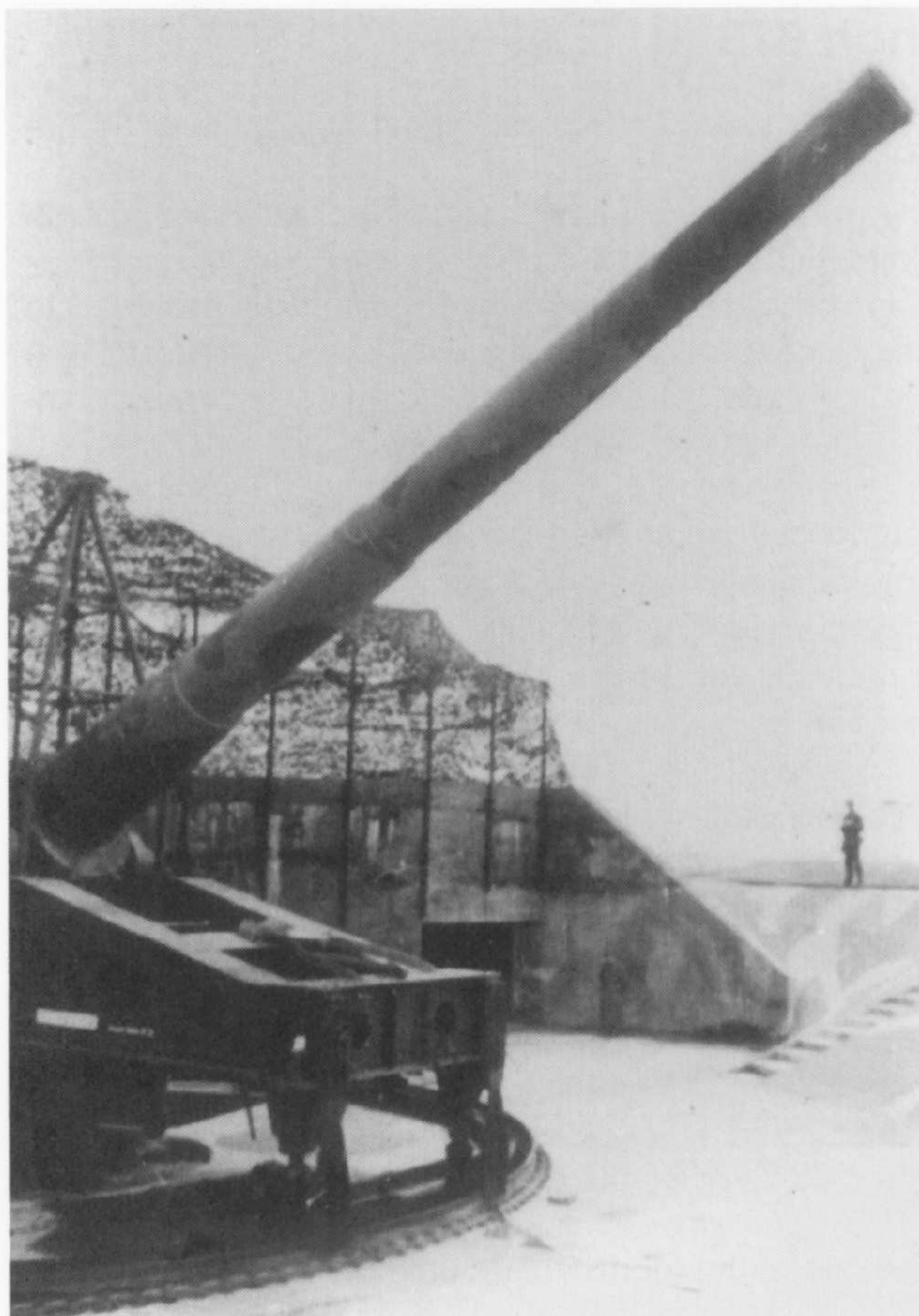
The barrel of the 34 cm Kanone 675 (f) at its greatest elevation of +42 degrees. Camouflage nets have been drawn over the bunker and the rear part of the gun.
